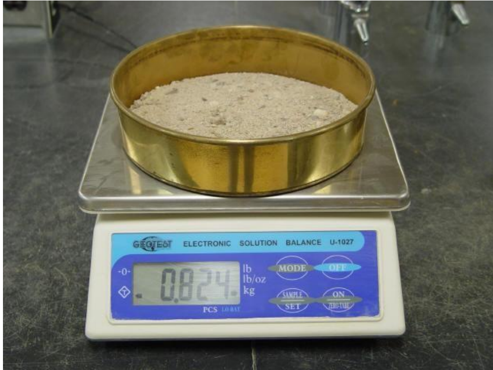
Fig: Illustrates Sieve Analysis test procedure
